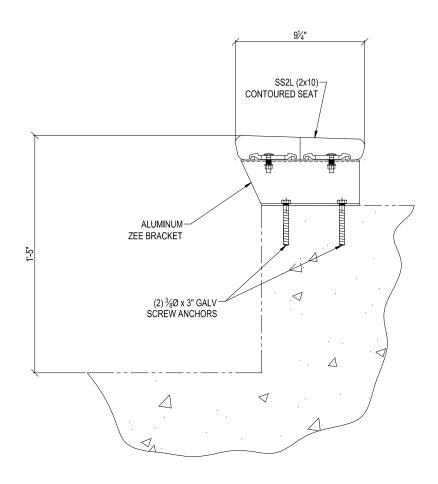
TREAD MOUNTED SEAT BRACKET W/ SS2L SEAT ATTACHED TO CONCRETE
